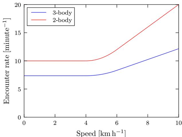
FIGURE 6.1. The 2- and 3-body encounter rate as a function of the reference body’s speed, and where the other bodies’ velocity distribution is made up of two rectangular functions with widths  $w$  around  $\pm V$ . For the purpose of this plot we assumed  $V = 5 \text{ km h}^{-1}$ ,  $w = 2 \text{ km h}^{-1}$ ,  $n = 120 \text{ km}^{-1}$  (representing a mildly busy street in Budapest), and  $\epsilon = 0.5 \text{ m}$  (representing a lower limit on comfortable personal space).
