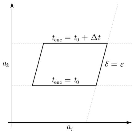
FIGURE 3.1. For the case where the reference body is  $i$  (largest speed in the positive direction), the area in  $a_j$ - $a_k$  space where the encounters satisfy  $\delta < \epsilon$  and  $t_0 < t_{\text{enc}} < t_0 + \Delta t$  is a parallelogram as shown.
